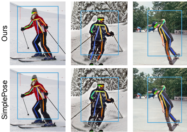
Figure 5: Qualitative comparison on truncations. Top: RLE. Bottom: Heatmap-based SimplePose. Only the contents inside the bounding boxes (blue) are fed to models.
